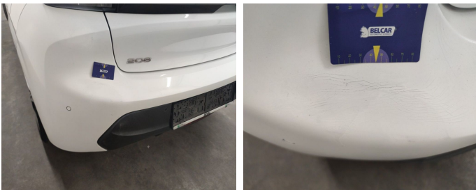
Bumper Rear // Repair & Painting-cracked
