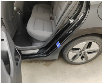
Rocker Panel Right // Smart Repair Medium-scratch + dent
