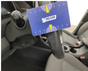
Dashboard / Steering Wheel / Replace-worn
