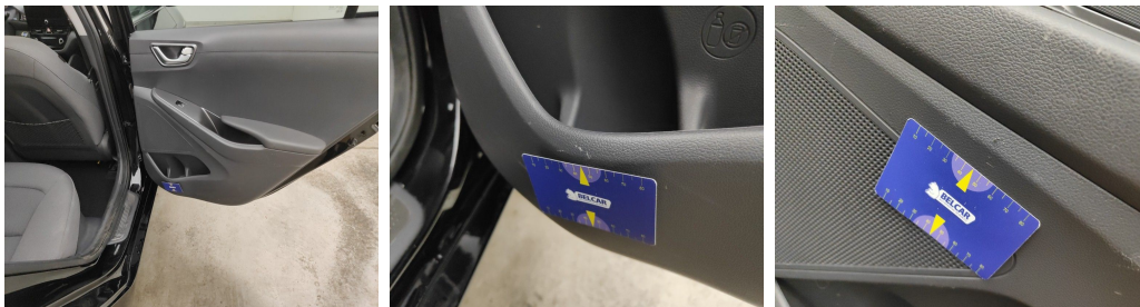
Rear Right Door Interior Coating // Replace Completely-scratch
