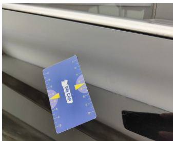
Door Rear Right // Repair & Painting-scratch + dent
