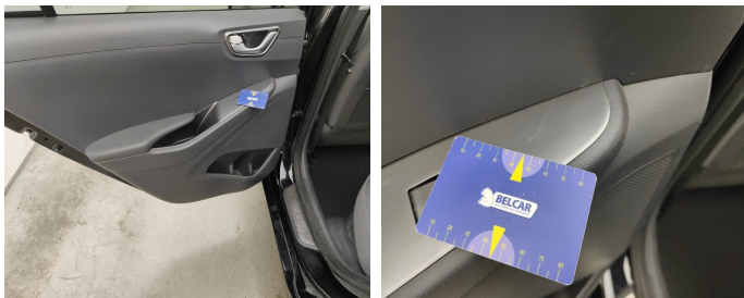
Rear Left Door Interior Coating // Repair-scratch
