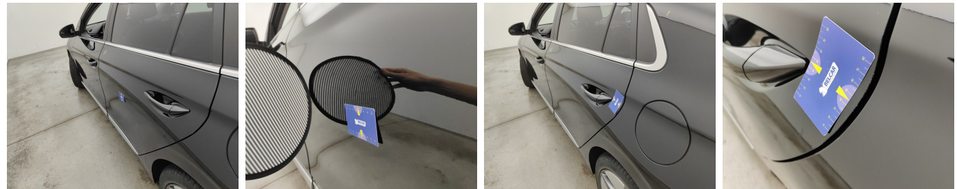
Door Rear Left // Smart Repair Medium-scratch + dent
