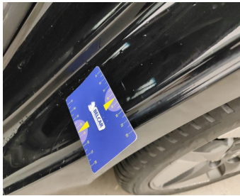
Rocker Panel Right // Smart Repair Medium-scratch + dent
