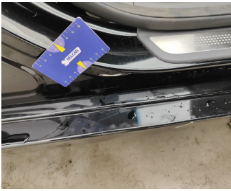
Rocker Panel Right // Smart Repair Medium-scratch + dent
