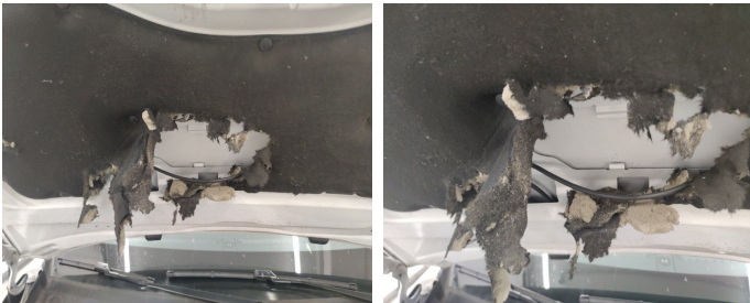
Front Bonnet / Insulation / Replace-cracked
