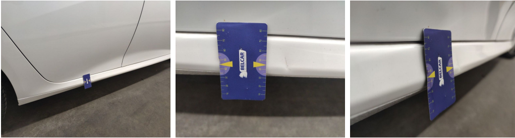
Rocker Panel Right // Repair & Painting-scratch + dent
