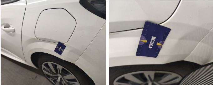
Wing Rear Left // Repair & Painting-dent
