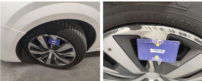
Wheel Front Left / Wheel Cover / Replace-scratch
