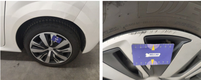
Wheel Rear Left / Wheel Cover / Replace-scratch
