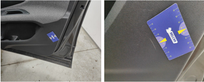
Front Right Door Interior Coating // Replace Completely-scratch
