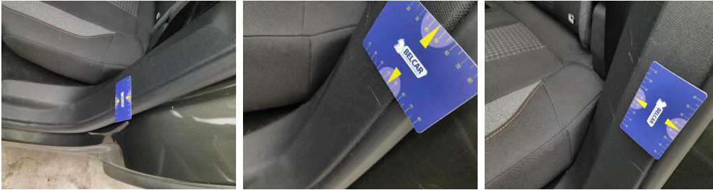
Seat Rear Left // Repair-scratch
