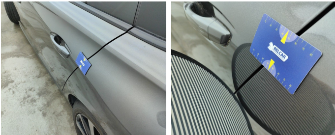
Wing Rear Left // Smart Repair Small-dent
