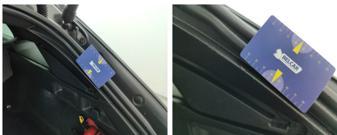
Trunk Compartment / Side Cover Right / Replace-scratch
