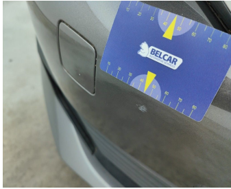
Bumper Front // Smart Repair Large-scratch
