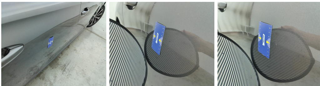
Door Rear Right // Repair & Painting-scratch + dent
