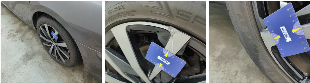
Wheel Alloy Rear Left // Replace-scratch + dent
