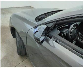
Side View Mirror Left // Painting-scratch
