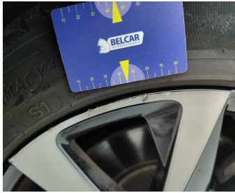
Wheel Two Tone Front Right // Repair-scratch
