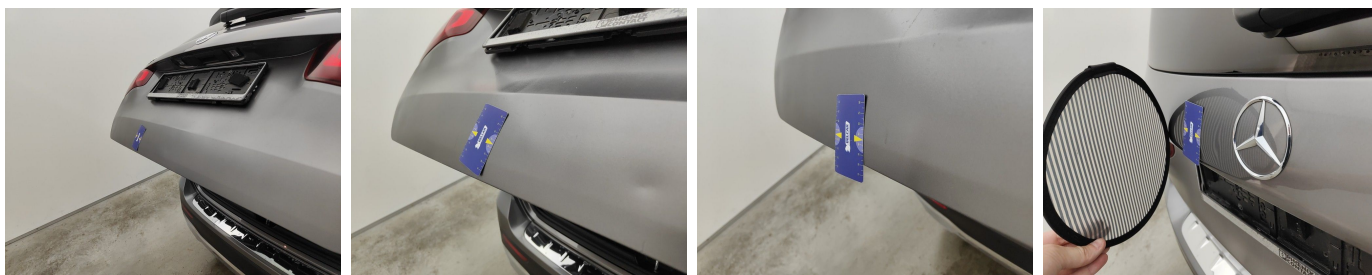
Rear Bonnet // Painting-bad repair
