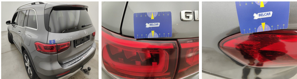
Light / Rear left / Replace-cracked
