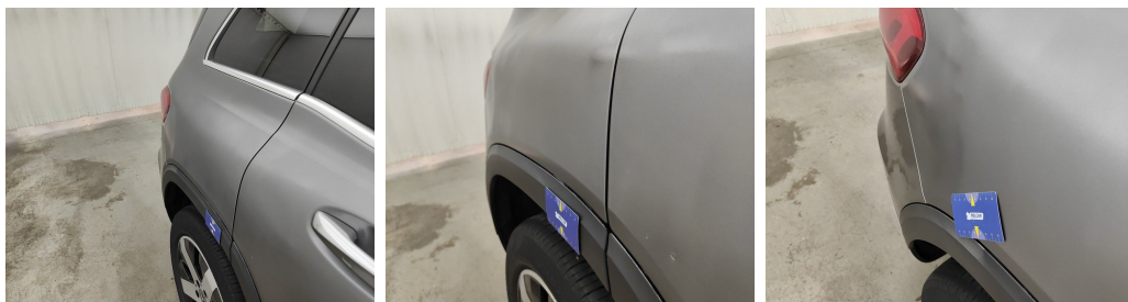
Wing Rear Right // Painting-bad repair
