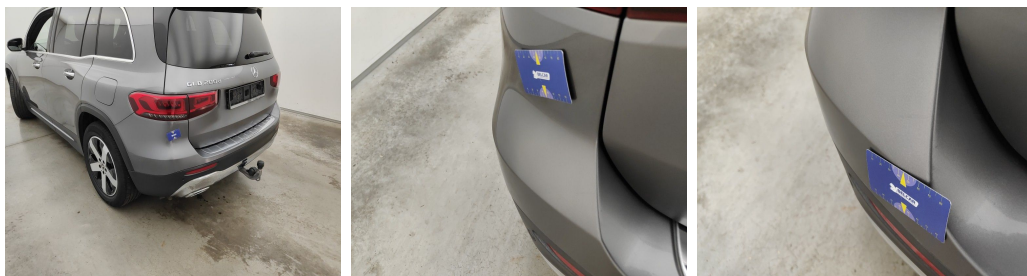
Bumper Rear // Painting-bad repair
