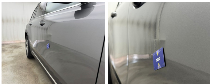
Door Front Right // Repair & Painting-bad repair
