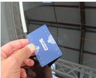
Rear Bonnet / Rear Window / Replace-scratch
