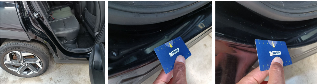
Rocker Panel Right // Smart Repair Medium-scratch + dent
