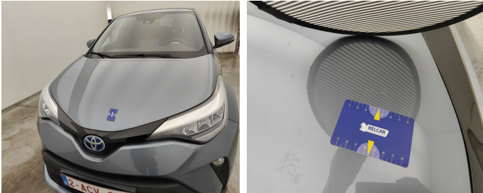
Front Bonnet // Repair & Painting-scratch + dent
