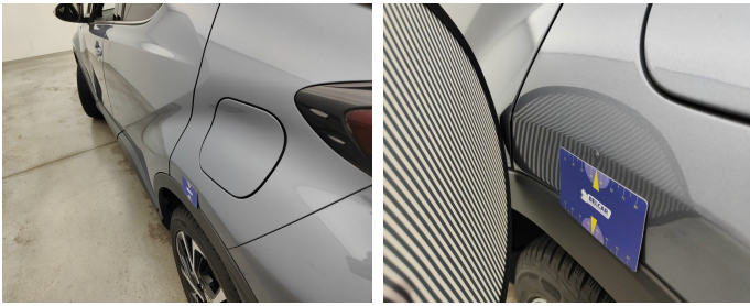
Wing Rear Left // Repair & Painting-scratch + dent
