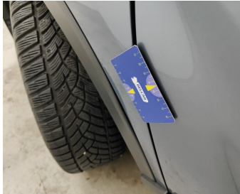
Wing Front Left / Trim / Replace-bad position
