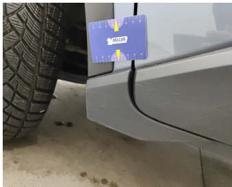
Rocker Panel Left / Cover Not Painted / Replace-scratch
