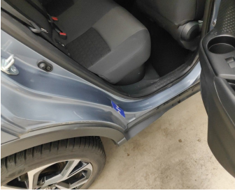
Rocker Panel Right // Polish-scratch
