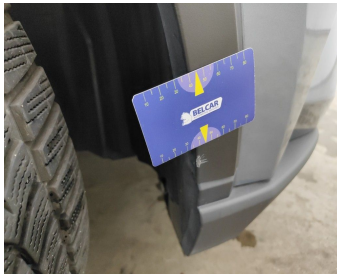
Wing Front right / Trim / Replace-scratch
