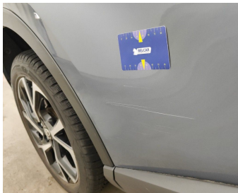
Wing Rear Left / Trim / Replace-scratch
