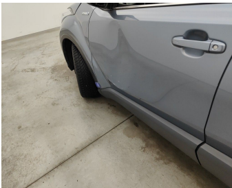
Rocker Panel Left / Cover Not Painted / Replace-scratch
