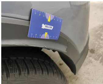
Wing Rear Left / Trim / Replace-scratch
