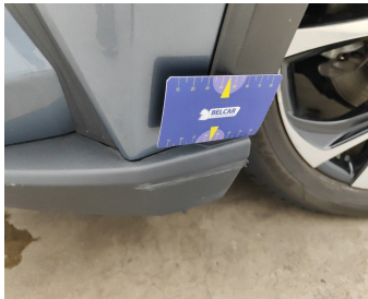
Bumper Front / Spoiler / Replace-scratch
