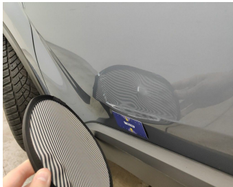
Wing Rear Right / Trim / Replace-scratch
