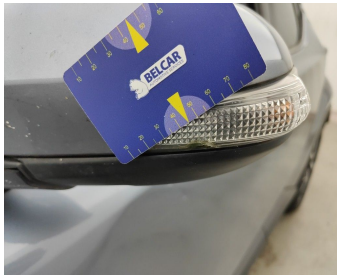
Side View Mirror Left / Direction Indicator / Replace-cracked
