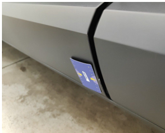
Door Front Left / Trim / Replace-scratch
