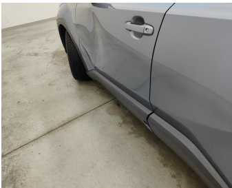
Door Front Left / Trim / Replace-scratch
