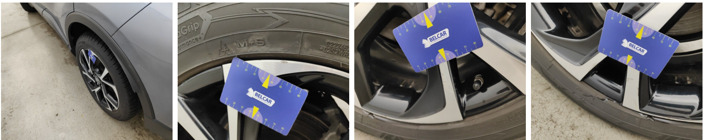
Wheel Two Tone Rear Left // Repair-scratch
