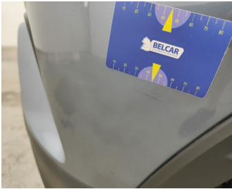
Bumper Rear // Painting-scratch
