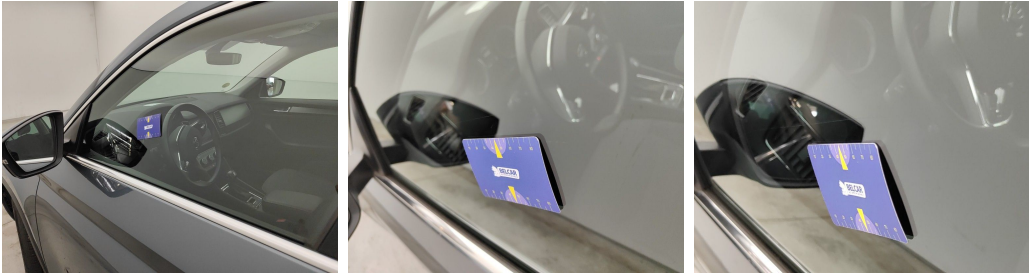
Door Front Left / Window / Replace-scratch
