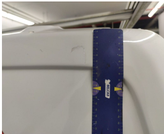
Rear Loading Door Right // Painting-bad repair
