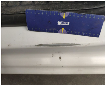
Rocker Panel Left // Smart Repair Medium-scratch
