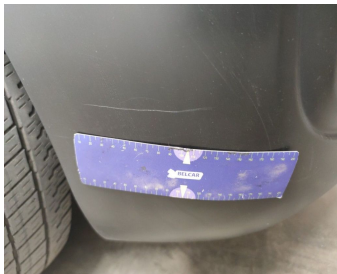
Bumper Front / Lower Cover Not Painted / Replace-scratch
