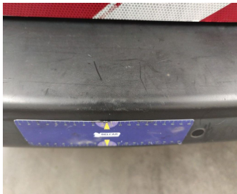
Bumper Rear / Lower Cover Not Painted / Replace-scratch
