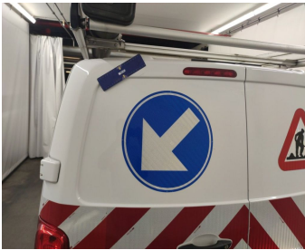
Rear Loading Door Left // Painting-bad repair
