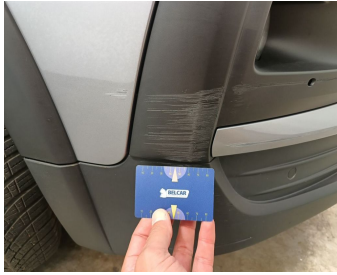
Bumper Front / Grid Right / Replace-scratch
