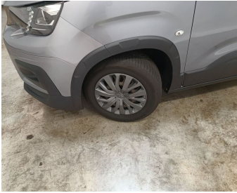
Wheel Front Left / Wheel Cover / Replace-scratch
