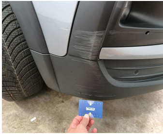
Bumper Front / Lower Cover Not Painted / Replace-scratch
