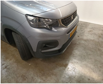
Bumper Front / Lower Cover Not Painted / Replace-scratch
