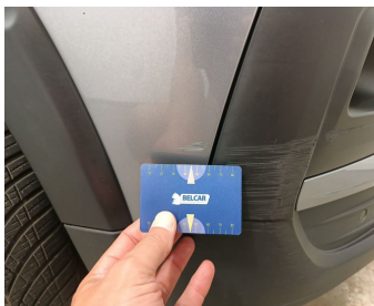
Bumper Front / Lower Cover Not Painted / Replace-scratch
