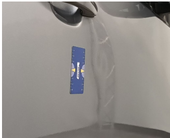
Door Front Right // Smart Repair Small-dent
