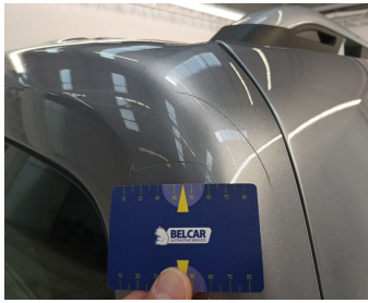
Rear Bonnet // Smart Repair Large-scratch
