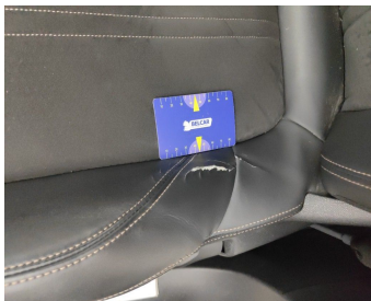
Seat Front Left / Bottom Coating / Replace-tear
