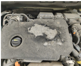
Front Bonnet / Insulation / Replace-tear
