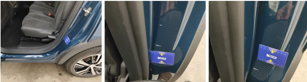
Rocker Panel Left // Smart Repair Medium-scratch + dent
