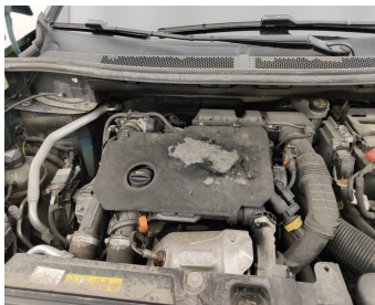
Front Bonnet / Insulation / Replace-tear
