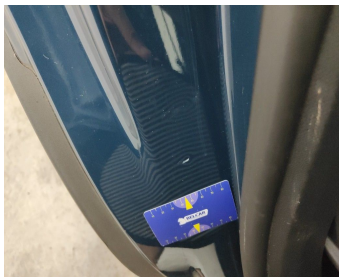
Rocker Panel Right // Smart Repair Medium-scratch + dent
