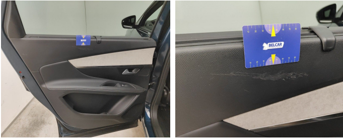
Rear Left Door Interior Coating // Replace Completely-scratch
