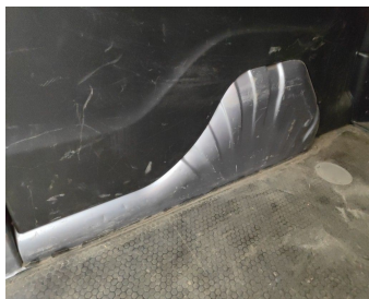
Trunk Compartment / Side Cover Left / Replace-scratch + dent
