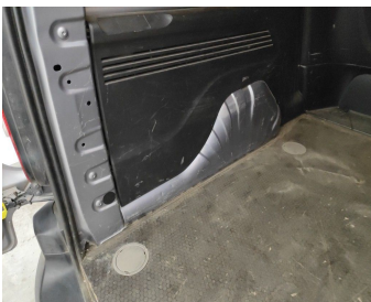
Trunk Compartment / Side Cover Left / Replace-scratch + dent
