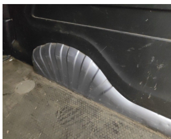
Trunk Compartment / Side Cover Left / Replace-scratch + dent
