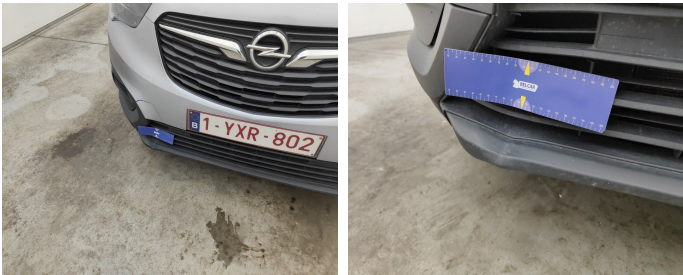
Bumper Front / Lower Cover Not Painted / Replace-dent
