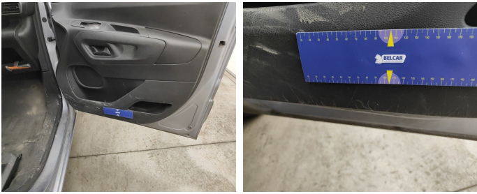
Front Right Door Interior Coating // Replace Completely-scratch
