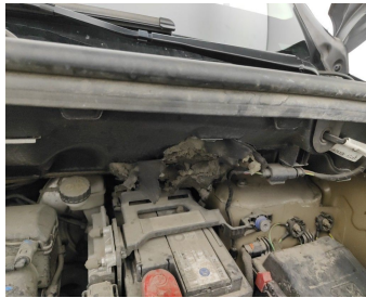
Front Bonnet / Insulation / Replace-tear
