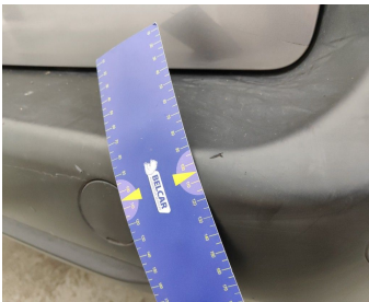
Bumper Rear / Lower Cover Not Painted / Replace-scratch
