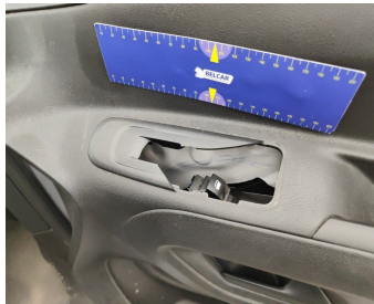
Front Right Door Interior Coating / Control Module / Replace-cracked
