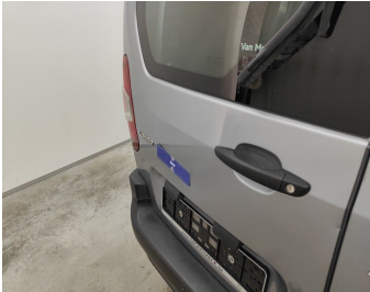
Rear Loading Door Left // Repair & Painting-scratch + dent
