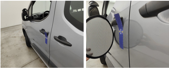
Door Front Left // Repair & Painting-dent
