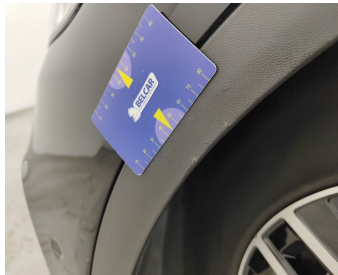
Wing Front Left / Trim / Replace-scratch
