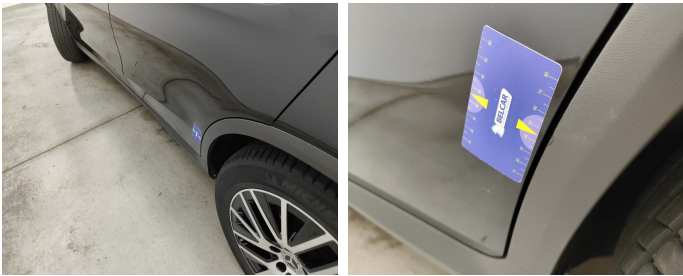
Wing Rear Left / Trim / Replace-scratch
