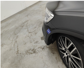
Wing Front Left / Trim / Replace-scratch
