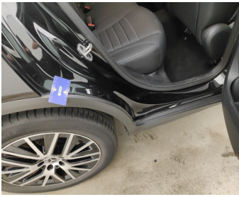
Rocker Panel Right // Polish-scratch
