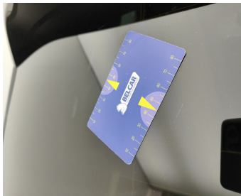
Rear Bonnet / Rear Window / Replace-scratch
